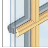
SIMULATED-DIVIDED-LIGHT WITH SPACER 7/8"
